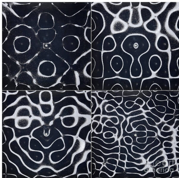
Figure 26.2: A chladni resonance image.
